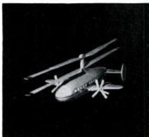
Rotor blades of Gyroliner model telescope inward to reduce drag in forward flight
